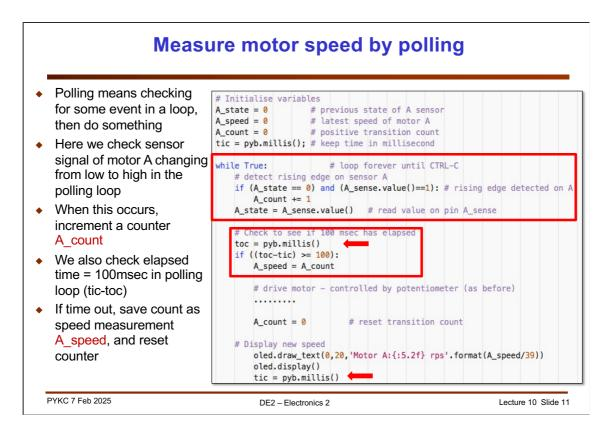
We measure the speed of rotation by counting the number of low-to-high transitions on one of the two Hall sensor signals.
