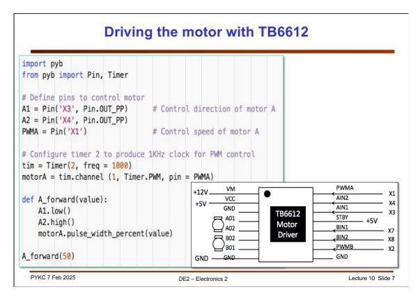
Exercise 1 of Lab 5 is just a revision from last year's Electronic 1 module. However, the TB6612 is NOT the same as the motor driver DRV8866 you used last year. TB6612 has two signals AIN1, AIN2 to control direction, and a separate PWMA signal to control the speed.
