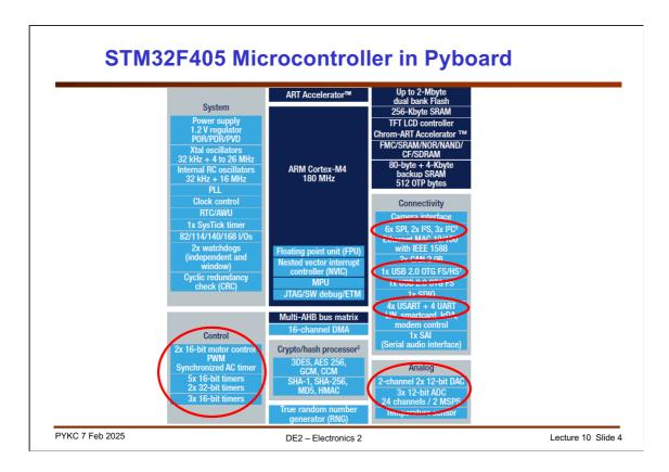
We are not only just using the ARM CPU. Instead, the Pyboard has a microcontroller as its main engine. This microcontroller, the STM32F405 is made by ST Micro, and here is an overview block diagram for this chip.
