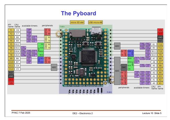
The Pyboard further add to the ST Micro chip by adding an accelerometer, a MicroSD card reader, all sort of power regulation and protection circuits.
