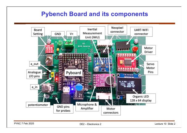
The Pybench hardware contains many modules. The heart of these is the **Pyboard**, which is a microcontroller board designed by the person who wrote MicroPython. You have already used the microphone/amplifier module, the IMU module and the OLED display module in previous Labs.
