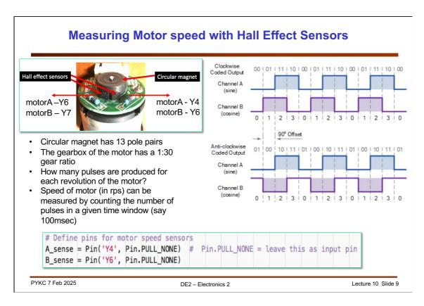
Next, we use the Hall Effect Sensors (two) on the motor to determine the speed of the motor and direction of the motor. The questions to ask yourself are:
