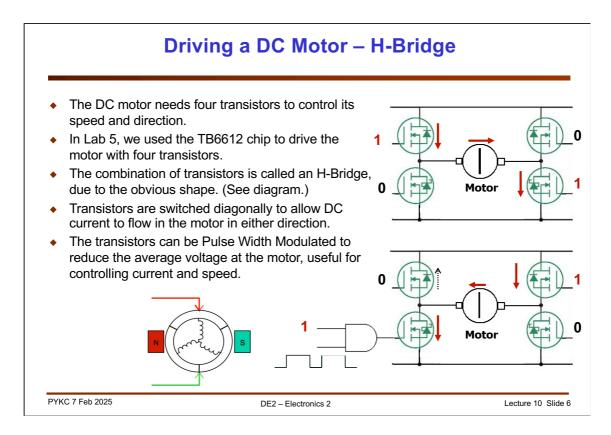
Since motor coils are essentially inductors, they have low DC impedances (resistance of the wiring). Hence when driving motors, we need to use a special driver chip.
